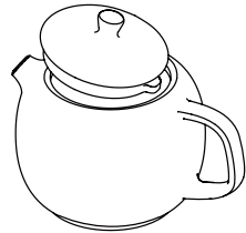
Couvercle muni d'un ergot anti-basculement. Lid with anti-tilt lug.
